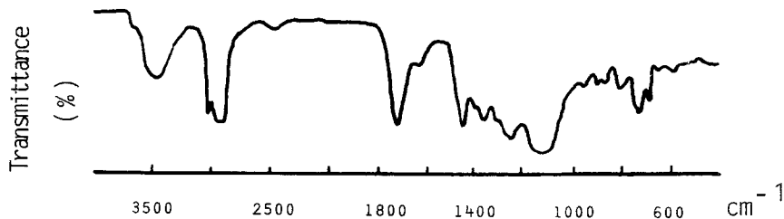
Figure 3. IR spectrum of poly(ε-pichlorohydrin) sample obtained using Ph 2 Zn-butanone system with a molar ratio butanone/Ph 2 Zn = 0.25.
